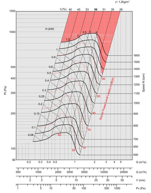
Performance certified is for installation type B - Free Inlet, Ducted outlet, Power rating kW does not include transmission losses, Performance ratings do not include the effects of appurtenances (accessories).
