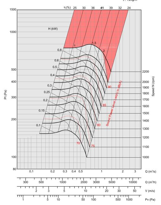
Performance certified is for installation type B - Free inlet, Ducted outlet. Power rating kW does not include transmission losses.
